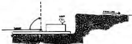
Figure 125. Countermine M31A1 target holding mechanism.
